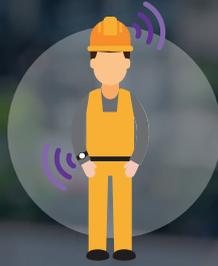
Worker and site productivity become measurable similar to a factory environment and allows optimisation; worker location used for safety management and interaction with autonomous machines
